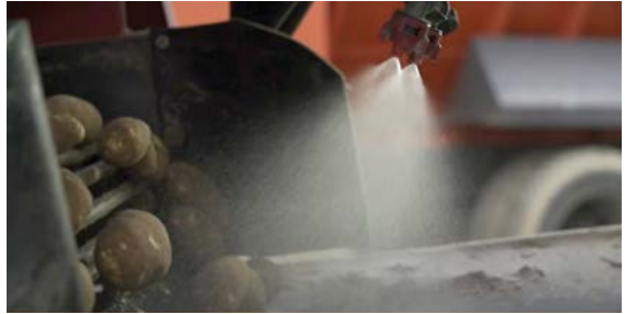
Overhead nozzles spray Stadium onto tumbling potato tubers.
