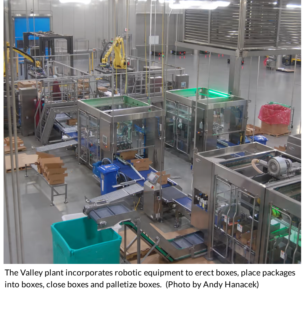
The Valley plant incorporates robotic equipment to erect boxes, place packages into boxes, close boxes and palletize boxes. (Photo by Andy Hanacek)
