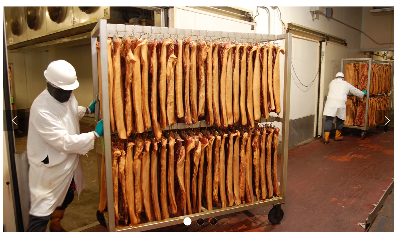
The monstrous smokehouse in the Denison, Iowa, plant holds 28 trees of product, equivalent to one truckload of bellies and the amount of trees they can fit in one blast cell.
