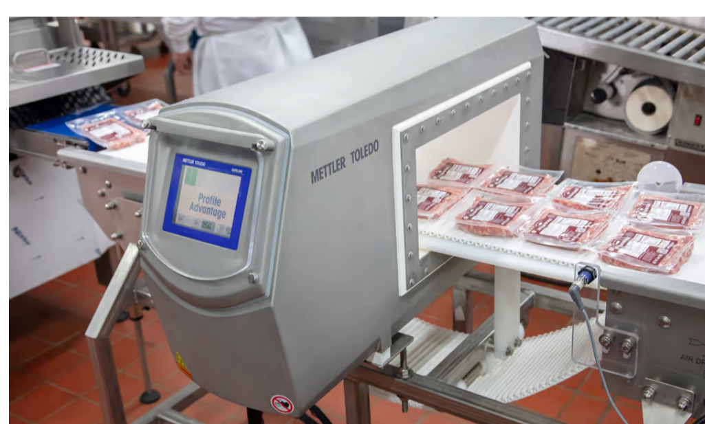
Longhini Sausage Co. rolls its newest metal detector from line to line to create an integrated quality-control system.
