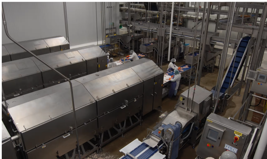
The processing floor of the Winesburg facility features automation to the extent that it doesn't seem with human action like a traditional chicken-processing plant might. Employees have been moved to safer, healthier roles while the machines do the ergonomically taxing work of handling and cutting the product.
