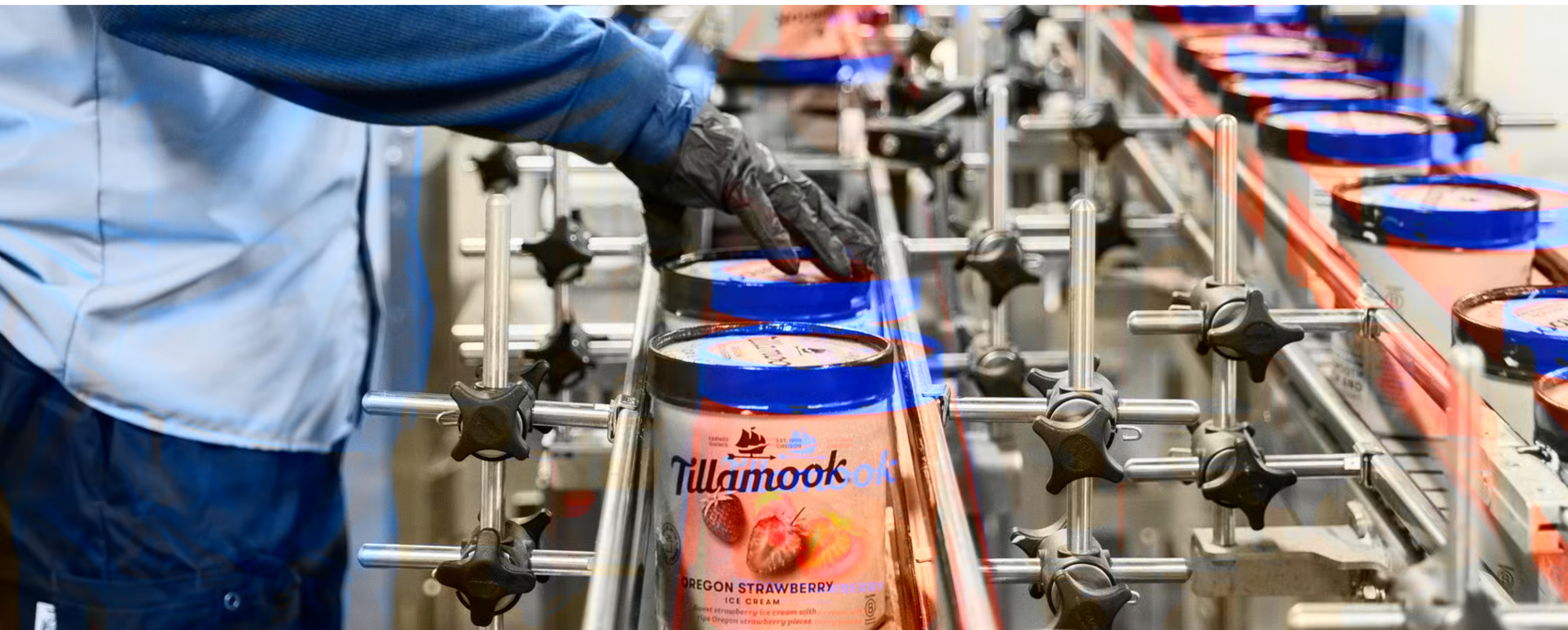
Tillamook makes ice cream cartons at its Decatur facility, with its forming machine making a new one every second. Photo courtesy of Tillamook
