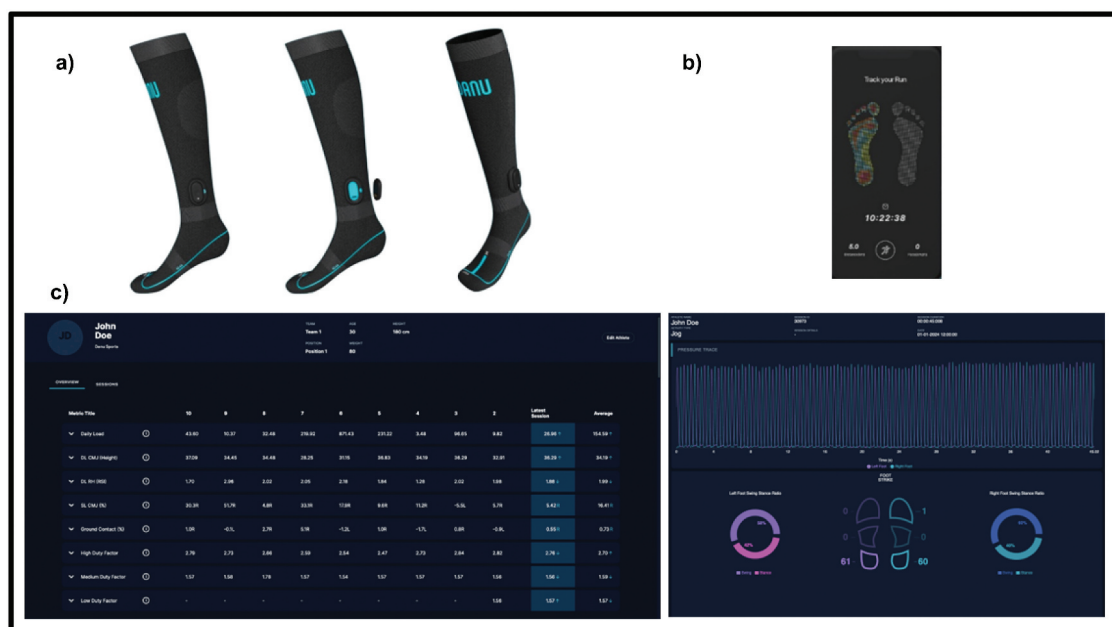
Figure 1. DANU human movement analysis system: a) DANU socks, b) smartphone or tablet application for data collection, c) data analytics on smartphone or tablet application (or computer).
