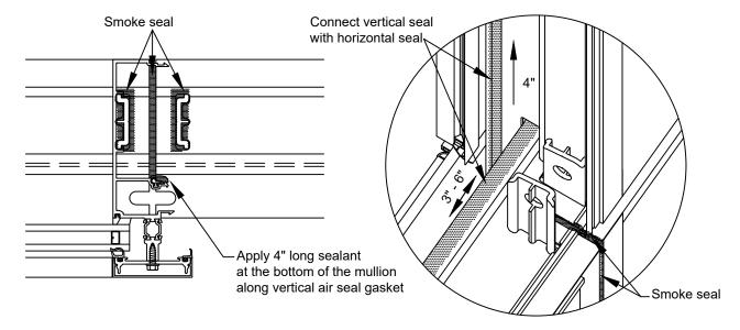
Install the next frame by lifting the frame 4" to 6" above previous frame to clear the sleeves and head horizontals. Move the next frame to the left to engage the outer mullion hooks; then rotate the next frame towards building to snap inner hooks; once snapped, slide the next frame down to engage horizontal air seal at stack joint.
