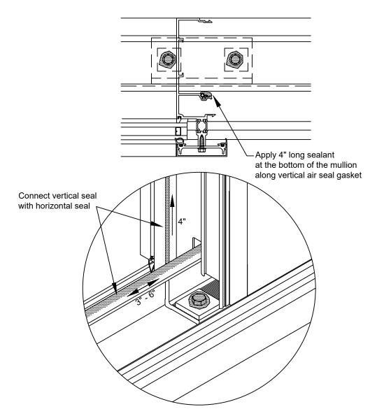
Install the next frame by lifting the frame up to clear the starter sill. Move the next frame to the left to engage the outer mullion hooks; then rotate the next frame towards building to snap inner hooks; once snapped, slide the next frame down to engage horizontal air seal at stack joint.
